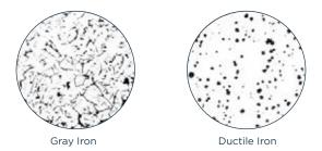
These photomicrographs compare the microstructures of gray iron and Ductile Iron. Note the relative continuity of the matrix exhibited by the Ductile Iron (right).
