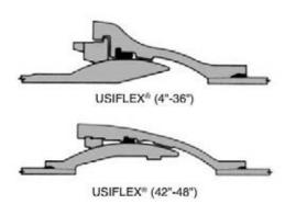
There are several methods of installing ball and socket Ductile Iron Pipe. It can be assembled in sections of three or four lengths, either on shore or on the deck of a barge, attached to a "strongback," and lowered to the stream bed where divers connect the sections. (Ball and socket pipes use joints with positive locking devices.) Ball and socket pipe can also be assembled on a chute affixed to the side of a barge and lowered into position as assembly progresses.
