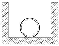
**Type 1\*** Flat-bottom trench.<sup>+</sup> Loose backfill.
