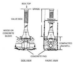
Valves can be placed in concrete or masonry vaults or buried in the soil with a valve box, or other device to allow access and operation, placed over the valve operator. All valves with exposed gearing should be installed in a vault. Access manholes should be large enough to allow removal of the valve if future replacement is necessary.
