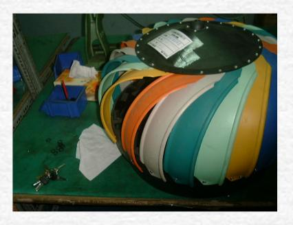
Painted black, Absorbing heat as much as possible to enhance the chimney effect by increasing  $\Delta T$ .
